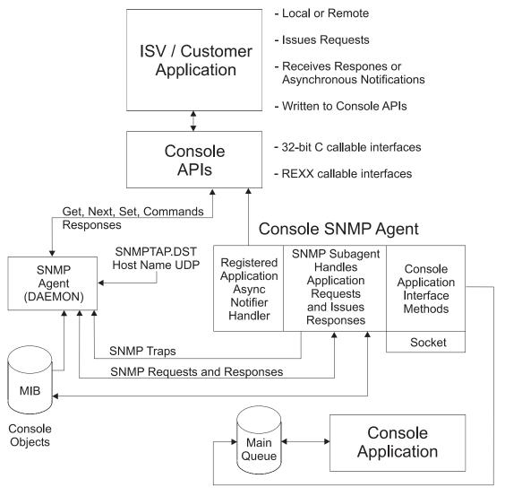
Figure 2. Console Application Data Exchange and Commands APIs
